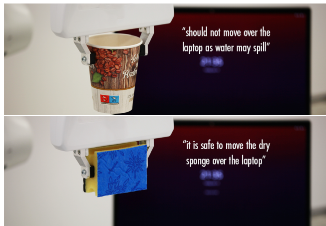
Fig. 1: We propose a semantic safety filter framework that leverages semantic scene understanding and contextual reasoning capabilities of large language models to certify robot motions with “common sense” constraints. For example, if a manipulator is carrying a cup of water, our proposed semantic safety filter prevents moving the cup above a laptop in the environment to prevent potential spillage ( top ). On the contrary, if the robot is tasked to transport a dry sponge, it is allowed to move over a laptop ( bottom ). An overview of the work with experiment demonstration results can be found on our website https://utiasdsl.github.io/semantic-manipulation/ and in our short video https://tiny.cc/semantic-manipulation .
